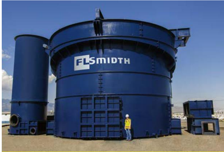
Şekil 2.17. SuperCell ® 600 m 3 (Courtesy FLSmidth)
