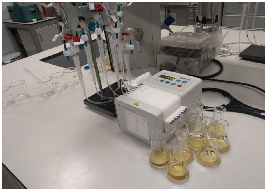
Figure 6.2. Photographs for biosorption of Pb(II) ions by the continuous system in apple juice
