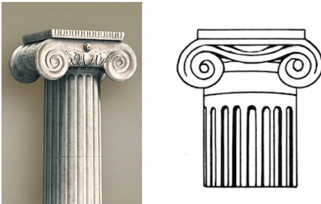
Figure 5.16. Ionic order drawings: a) 3D model, b) 2D drawing (URL4, arkeofili).
