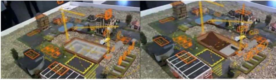
Figure 4.14. Observation of the construction site process with the MAR to plan Virtual Construction Work Sites application (Abboud, 2014).
