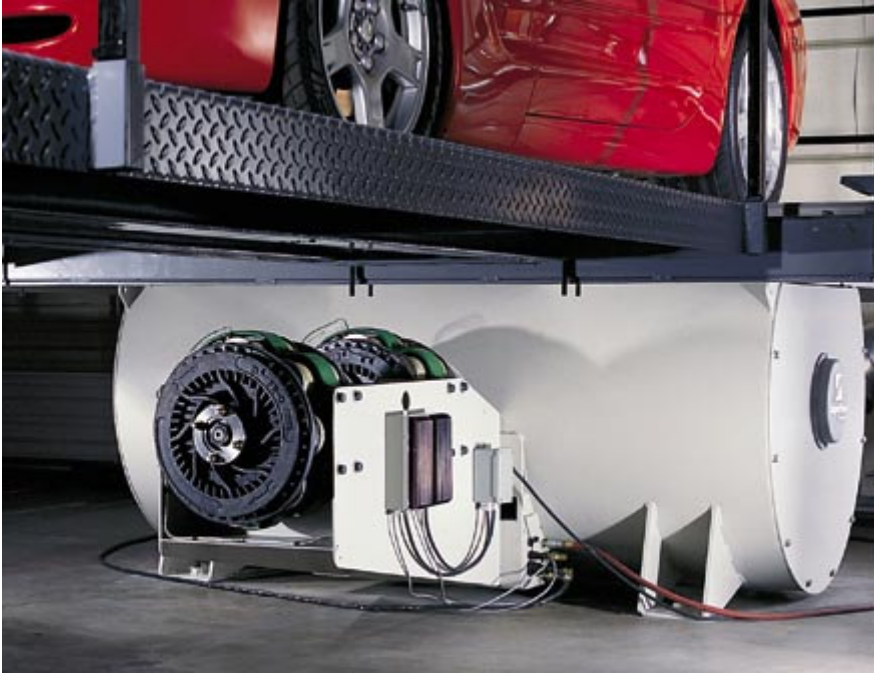
Őekil 2.6.a Őasi dinamometresi- gũ emici - Dual Eddy ( http://www.superflow.com/ )
