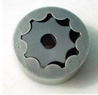
Şekil 3.3. Gerotor pompa ( http://extreme.infomagic.net/static/SmGerotor.jpeg )
