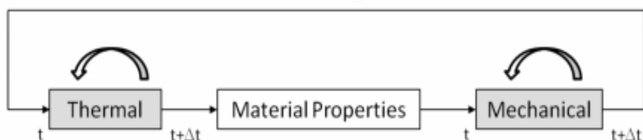
Figure 2.15. Thermal and Mechanical behavioural relationship in a coupled thermo-mechanical model.
