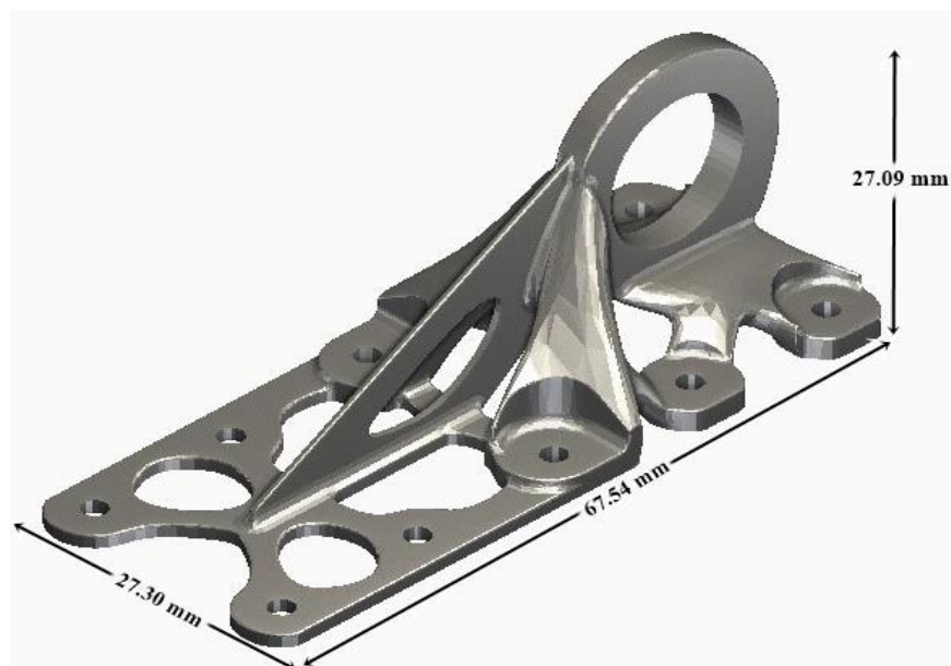
Figure 3.2. CAD part used for the simulation.
