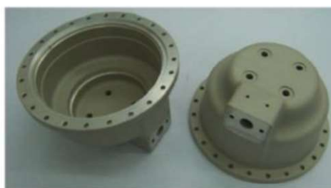
Figure 2.2. Air conditioning system made of magnesium alloy WE43 for aircraft (Dziubińska et al., 2016).
