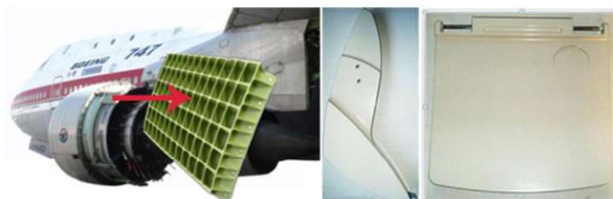
Figure 2.1. Examples of application for magnesium alloys in Boeing 747: wing and seat components (Dziubińska et al., 2016).
