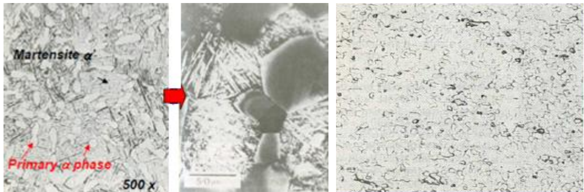
Şekil 4.6. a) Hekzagonal \alpha' b) Lenticular \alpha' c) Ortorombic \alpha'' (Lütjering & Williams, 2007).
