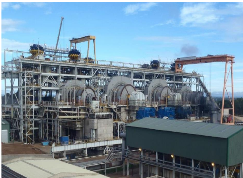
Figure 5.8. Milling circuit showing the SAG and ball mills.
