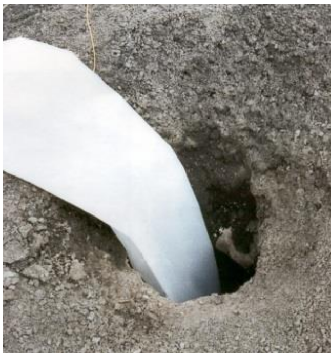
Figure 5.4. Use of blast hole liner to prevent the contact of ammonium nitrate and sulphides.
