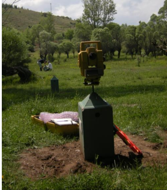
Şekil 8.2 Topcon Marka GPT 8005a model Total Station
